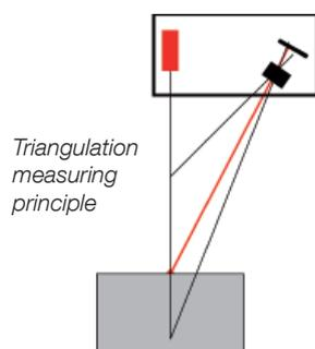
By analysing the position with the highest light intensity on the CCD line and based on the fixed geometrical relationship (triangulation), the position can be converted to a distance with the help of the calibration curve stored in every measuring head.
