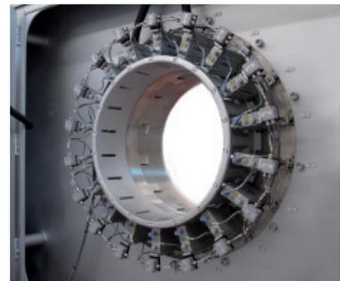
*18-channel diameter profile measuring system*
