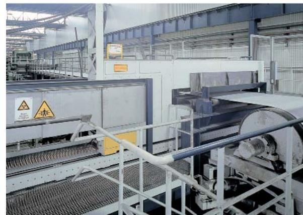
Three-head thickness gauge (traversing)
