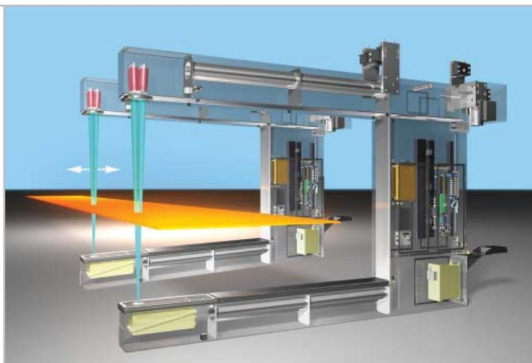
*Twinset thickness and profile measuring frame*
