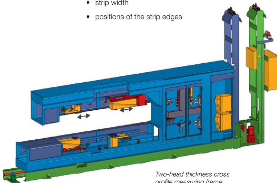
*Two-head thickness cross profile measuring frame*
