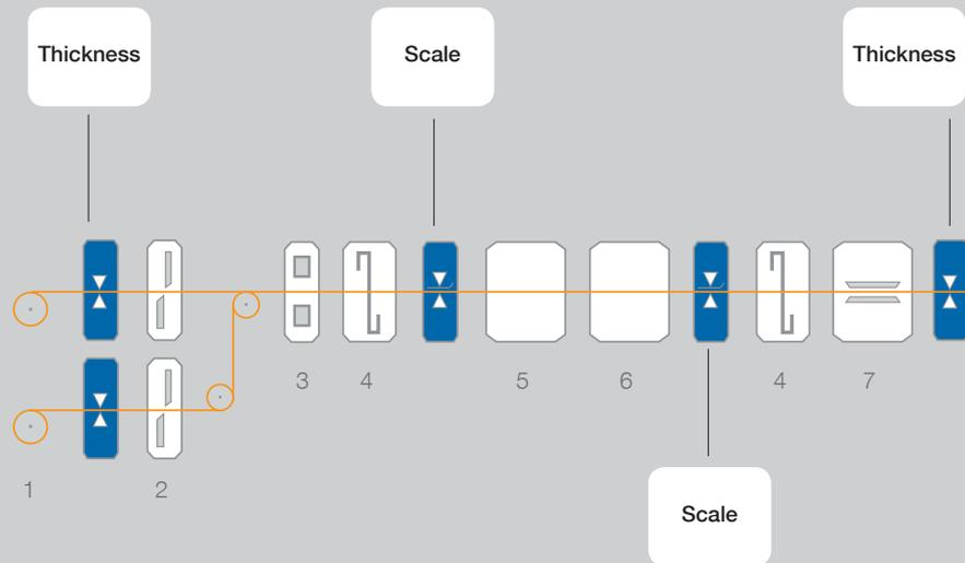
*Example of a typical configuration of a cold rolling tandem mill*
