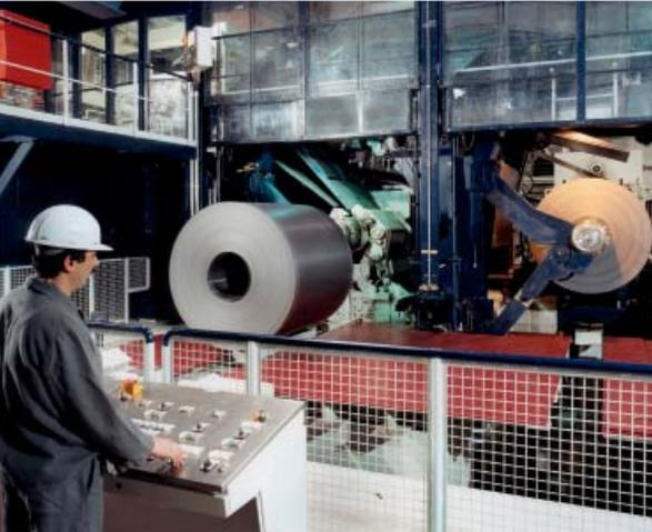
Cold rolling tandem mills are usually built as continuous lines with direct connection to pickling lines.
