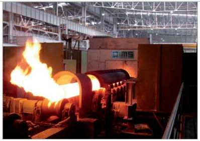
Diameter profile measuring system in a PQF® mill
