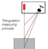
By analysing the position with the highest light intensity on the CCD line and based on the fixed geometrical relationship (triangulation), the position can be converted to a distance with the help of the calibration curve stored in every measuring head.
