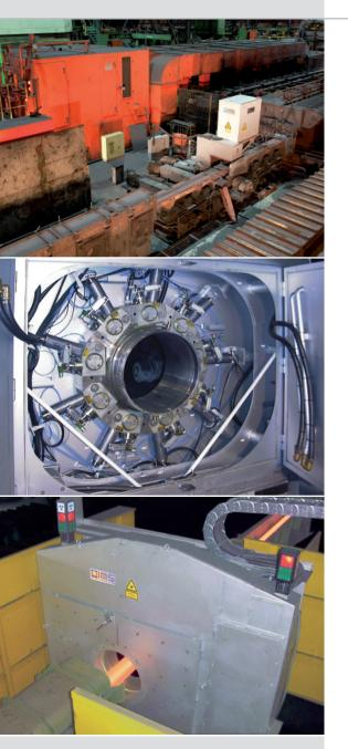
From top to bottom: Stretch reducing mill – 1-channel system Internal view sources/detectors – 9-channel system Exit sizing mill – 9-channel system
