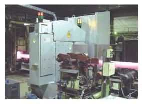
Multi-channel measuring system at entry to walking beam furnace
