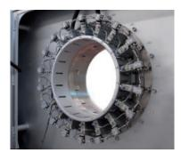
18-channel diameter profile measuring system
