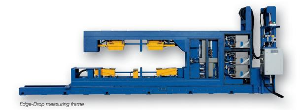
Material thickness is measured in the centre and at the edges of strip by a three-head measuring frame equipped with three x-ray tubes, each with a separate detector unit. The centreline detector unit has two to four detectors and the two detector units on the outside have an array of four to 22 detectors depending on the application.
