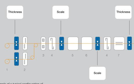
Example of a typical configuration of a cold rolling tandem mill
