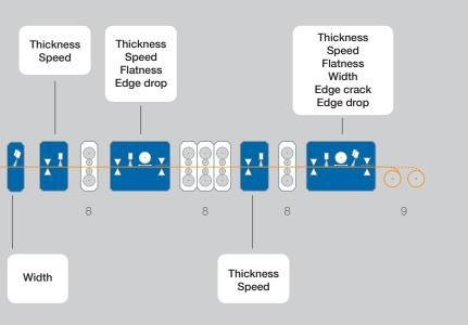
For optimum control of the process parameters and quality assurance, the following measuring systems are integrated in a combined pickling/ tandem line:
