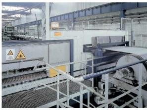
Three-head thickness gauge (traversing)
