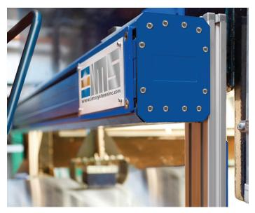
The IMS-CCS Width Gauge uses the latest optical measuring technology to take real-time, point-to-point measurements that help to ensure superior strip quality.
